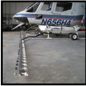
(Left) Helicopter used for aerial herbicide treatments by Helicopter Applicators, Inc.. (Center) Spray-boom and Microfoil spray nozzles used in helicopter precision applications of herbicides to control invasive vegetation in Loxahatchee NWR and other areas in south Florida. (Right) Specialized herbicide mixing truck with helicopter landing pad mounted above the water and mixing tanks.
