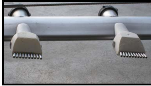
(Left) Helicopter used for aerial herbicide treatments by Helicopter Applicators, Inc.. (Center) Spray-boom and Microfoil spray nozzles used in helicopter precision applications of herbicides to control invasive vegetation in Loxahatchee NWR and other areas in south Florida. (Right) Specialized herbicide mixing truck with helicopter landing pad mounted above the water and mixing tanks.
