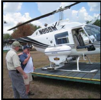
The Lee County Mosquito/Hyacinth Control District maintains a fleet of helicopters and C-47 fixed winged planes to implement required control efforts for large-scale mosquito abatement and invasive weed management activities. In the photo above, Lee County staff demonstrated an aerial spray application for mosquito control using a Huey helicopter.
